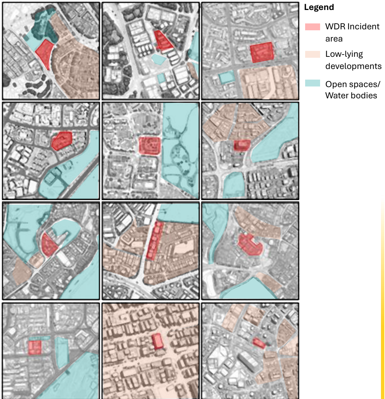
Figure 4: Diagrammatic study of typical site conditions leading to wind-driven rain
